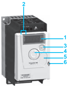
ATV 12H075M2 with door on front panel closed with protective cover 5: STOP/RESET and RUN buttons not accessible
