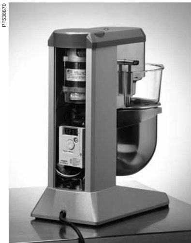
ATV 12 controlling a mixer
